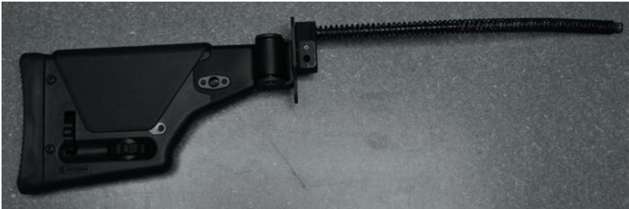
The butt stock assembly is comprised of the stock itself with the hinge mechanism, receiver end cap, buffer and recoil springs. It is pinned to the receiver by a single locating pin of the detent type.
